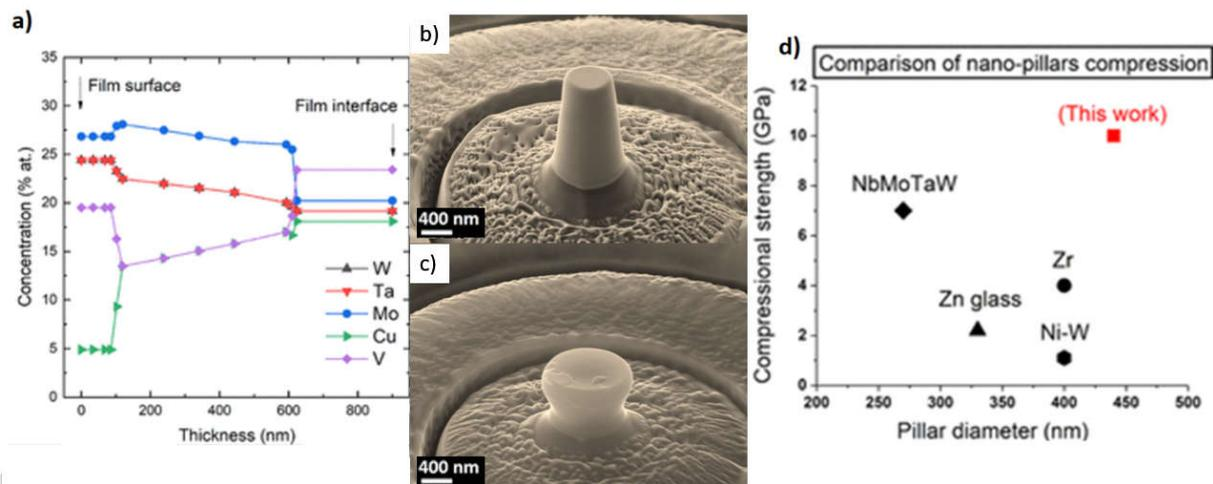
Fig. 2. a) Concentration of elements b) milled nano-pillar before compression c) milled nano-pillar after compression d) compressional strength results
