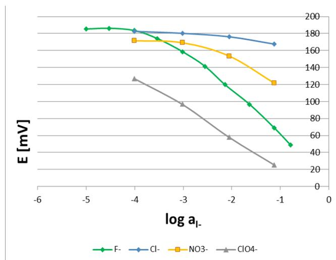
Fig. 2. Selectivity plot of the ready electrodes with dithizon-silver complex inside the membrane
