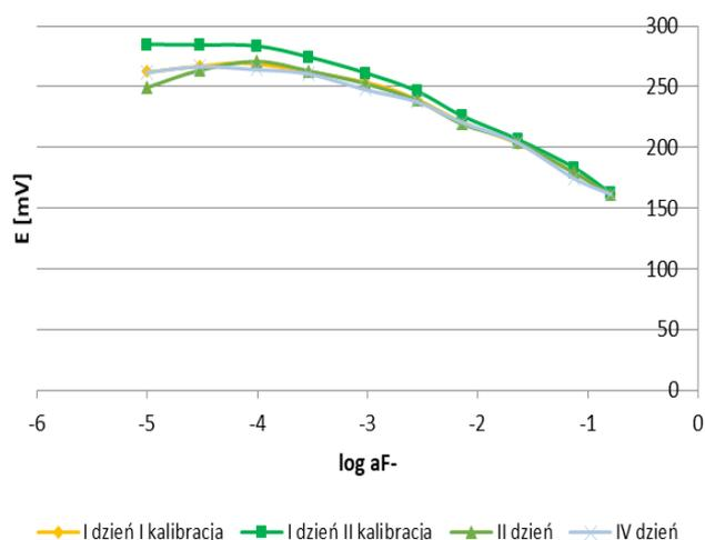
Fig. 1. Calibration curve of the electrodes with dithizon-silver complex inside the membrane
